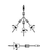
Filling leads with Female Large Screw adapter to connect with single EVA bags and multilayer bags for gravity filling procedures
